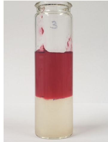
Fig. 2. An example of an experiment with the colored gelatin poured in. Note that some of the gelatin has stuck to the walls in this case because the colored gelatin was close to being too cool to pour smoothly.
